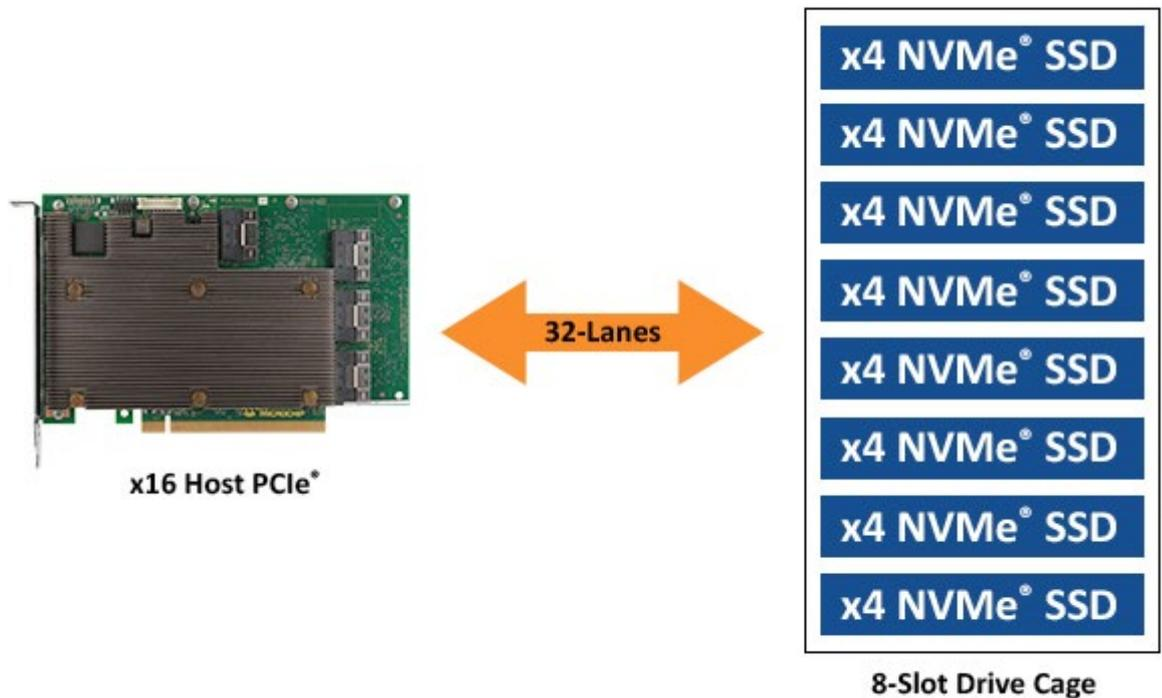
One adapter delivers maximum performance to eight ×4 NVMe SSDs in single standard drive cage.
