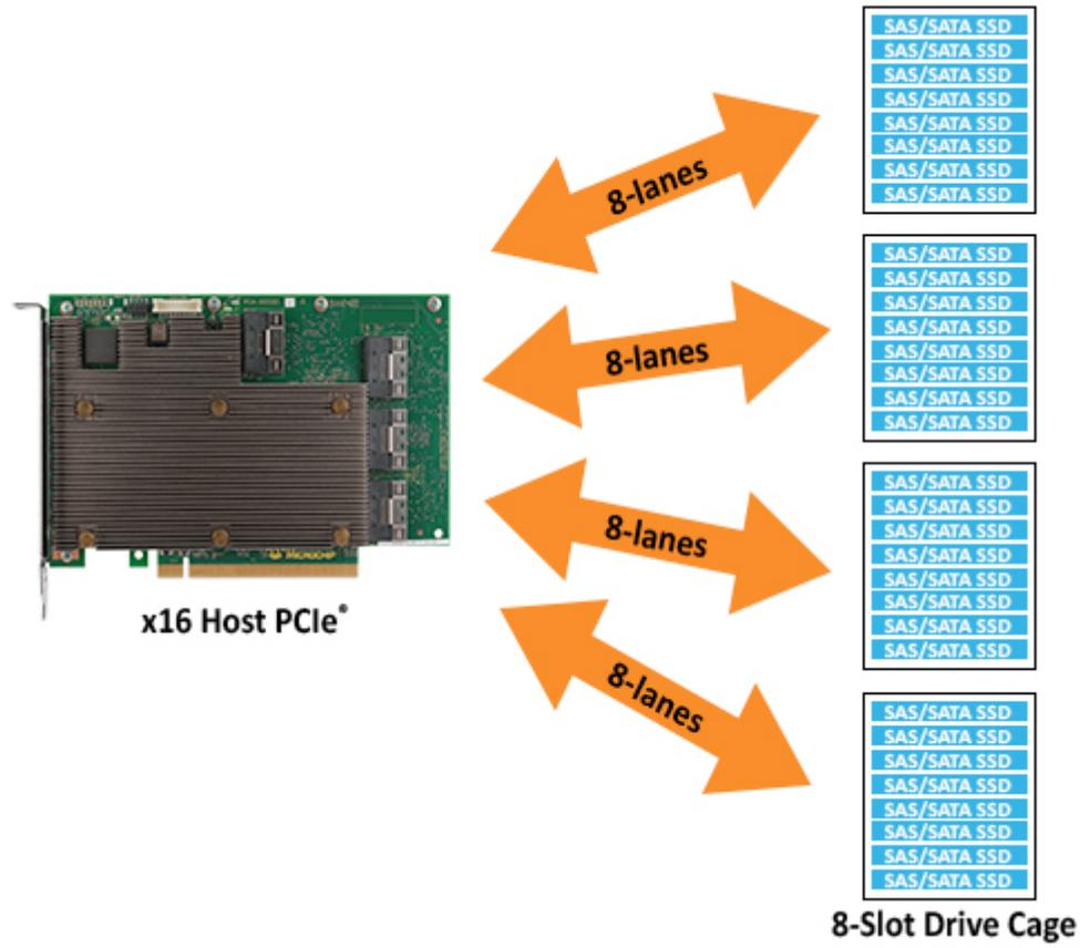
One Adapter delivers maximum fanout for 32 SAS/SATA devices across four standard drive cages
